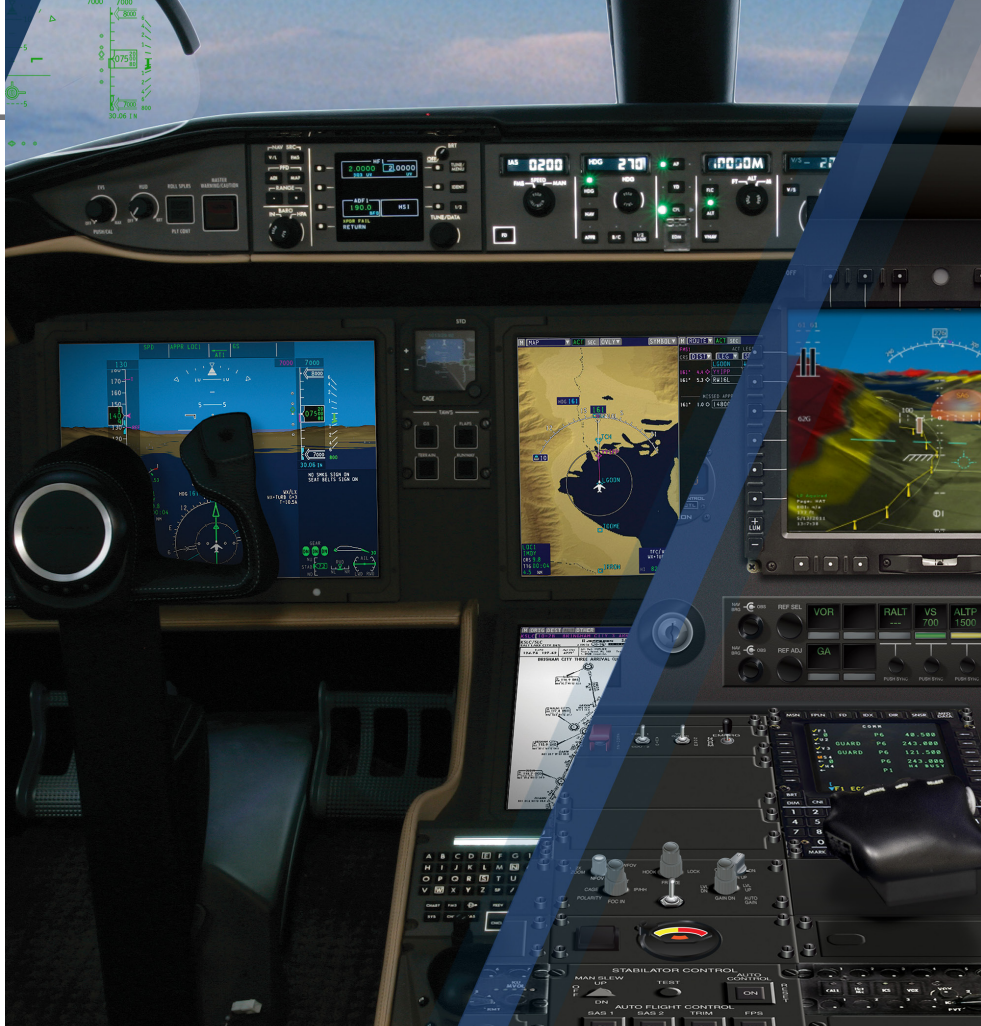
A Pro Line Fusion Synthetic Vision system developed by Rockwell Collins for the Bombardier Global 5000 business jet's flight deck has been adapted for the MH-60 Black Hawk helicopter. (Photo courtesy of Rockwell Collins)
