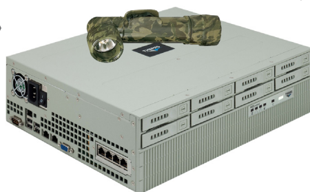
Figure 1 | Themis Computer's RES-mini SFF high-density servers aim for a high functionality-to-size ratio by managing the thermal challenges that come with Intel Xeon E5 1600 and 2600 devices.
