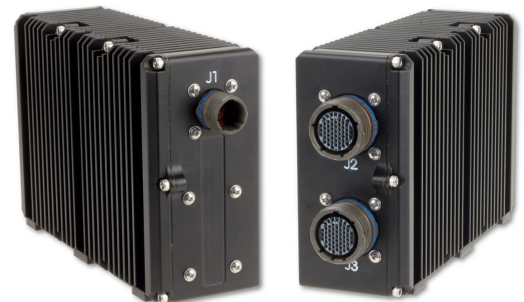
Figure 2 | The XPand6000 Series from Extreme Engineering Solutions (X-ES) attaches the die of the processor directly to the chassis wall to maximize natural conduction cooling.
