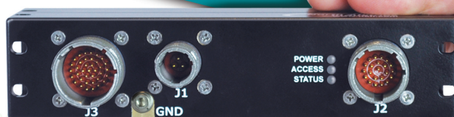
The Nano Interface Unit (NIU1) measures only 6.5"W x 1.5"H x 1.6"D.
