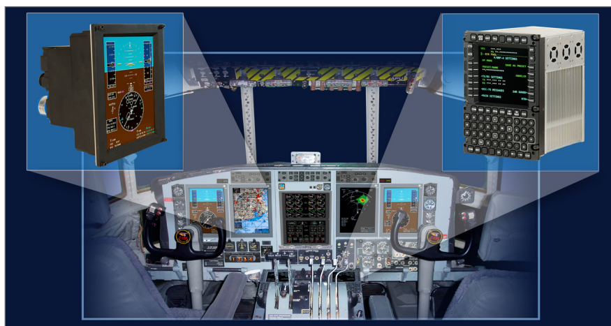
Figure 1 | The Navy's modernization of the C130-T's avionics by Lockheed Martin requires conformance to the FACE standard for software.
