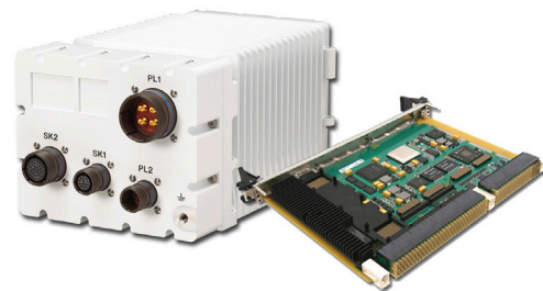
Figure 1 | Curtiss-Wright Controls Defense Solutions' MPMC-9335 3U VPX Mission Computer and its VPX6-187 6U VPX SBC are examples of FACE Candidate Hardware that can host FACE Candidate Software.
